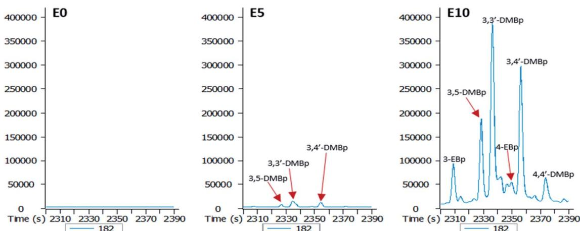
Fig. 7 Partial  $m/z$  182 mass chromatograms of the E0, E5 and E10 leachates showing identification of  $C_2$  alkylbiphenyls [DMBp: dimethylbiphenyl; EBp: ethylbiphenyl; E0: unblended diesel fuel; E5: diesel fuel containing 5% ethanol (v/v); E10: diesel fuel containing 10% ethanol (v/v)].
