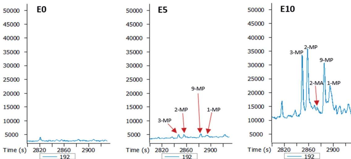
Fig. 6 Partial  $m/z$  192 mass chromatograms of the E0, E5 and E10 leachates showing identification of methylphenanthrenes (MP) [E0: unblended diesel fuel; E5: diesel fuel containing 5% ethanol (v/v); E10: diesel fuel containing 10% ethanol (v/v)].
