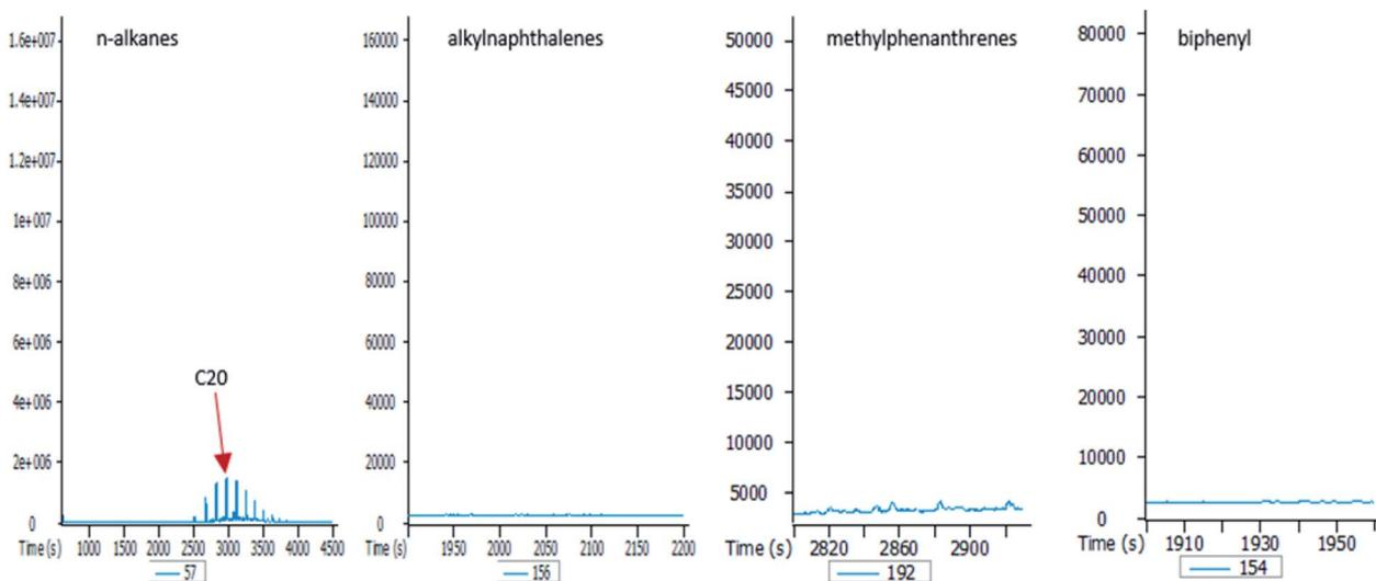
Fig. 8 Partial mass chromatograms ( $m/z$  57, 156, 192 and 154) of the E20 leachates, showing limited ( $n$ -alkanes) or no elution of diesel fuel hydrocarbons ( $C_{20}$  alkylnaphthalenes, methylphenanthrenes, biphenyl). E20: diesel fuel containing 20% ethanol (v/v).
