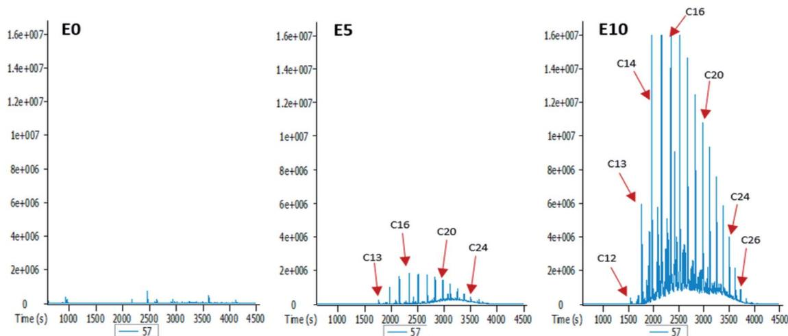
Fig. 4 Partial  $m/z$  57 mass chromatograms of the E0, E5 and E10 leachates, showing identification of a homologous series of  $n$ -alkanes [E0: unblended diesel fuel; E5: diesel fuel containing 5% ethanol (v/v); E10: diesel fuel containing 10% ethanol (v/v); Cx:  $n$ -alkanes containing  $x$  number of carbon atoms].
