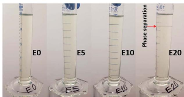
Fig. 1 Stability of four ethanol blends at 20 °C.
