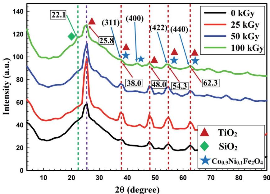
Fig. 5 XRD pattern showing the effect of gamma irradiation, with doses of 25, 50 and 100 kGy, on the crystal size of the prepared  $\text{Co}_x\text{Ni}_{1-x}\text{Fe}_2\text{O}_4/\text{SiO}_2/\text{TiO}_2$ ;  $x = 0.9$  nanocomposite, compared with the non-irradiated composite.
