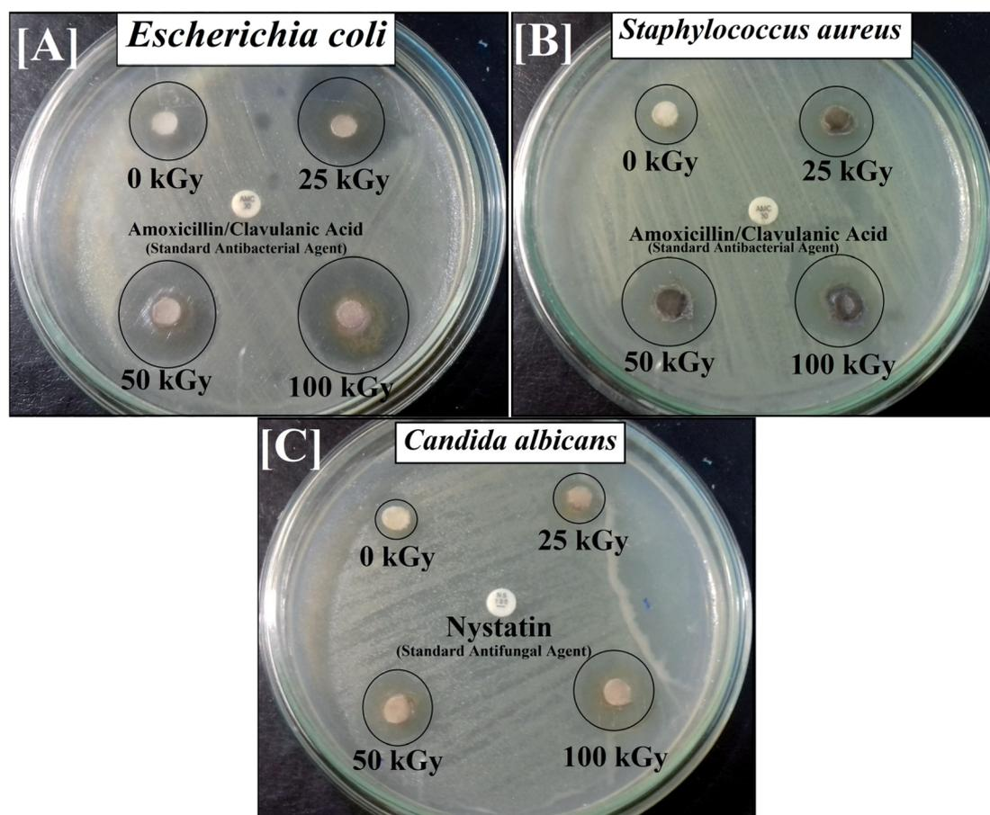
Fig. 4 Antibacterial and antifungal activities of gamma-irradiated  $\text{Co}_x\text{Ni}_{1-x}\text{Fe}_2\text{O}_4/\text{SiO}_2/\text{TiO}_2$ ;  $x = 0.9$  nanocomposite against pathogenic microbes for [A] *E. coli*, [B] *Staphylococcus aureus* and [C] *C. albicans*, measured as ZOI (mm).
