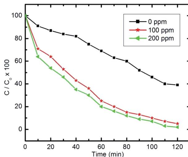
Fig. 15 Effect of H<sub>2</sub>O<sub>2</sub> on pyridine degradation (initial concentration of pyridine C<sub>0</sub> = 100 ppm, 50 ml, 10 mg of nanocomposite and pH 9).
