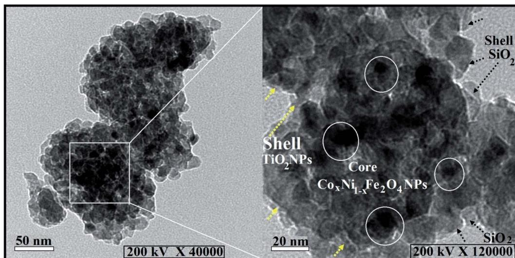
Fig. 1 HRTEM analysis of the prepared  $\text{Co}_x\text{Ni}_{1-x}\text{Fe}_2\text{O}_4/\text{SiO}_2/\text{TiO}_2$ ;  $x = 0.9$  hybrid nanocomposite concentric structure, where yellow and black arrows display the two shell layers and the white circles represent the core  $\text{Co}_x\text{Ni}_{1-x}\text{Fe}_2\text{O}_4$ ;  $x = 0.9$  NPs.
