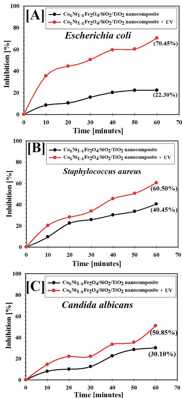
Fig. 6 Antimicrobial abilities of UV-irradiated  $\text{Co}_x\text{Ni}_{1-x}\text{Fe}_2\text{O}_4/\text{SiO}_2/\text{TiO}_2$ ;  $x = 0.9$  nanocomposite against different pathogens: [A] *E. coli*, [B] *S. aureus* and [C] *C. albicans*.
