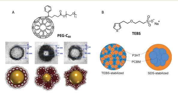
Fig. 7 (A) TEM image of a core-shell NP stabilized by PEG-C<sub>60</sub>, the core is composed of P3HT and the shell of PEG-C<sub>60</sub> micelles mixed with various amounts of PC<sub>61</sub>BM. Adapted with permission from ref. 37 (Copyright 2018 Wiley-VCH Verlag). (B) Scheme of the structure of P3HT:PC<sub>61</sub>BM stabilized by TEBS. Adapted with permission from ref. 38 (Copyright 2018 American Chemical Society).
