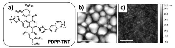
Fig. 14 (a) PDPP-TNT chemical structure. AFM images of (b) an as-spun PDPP-TNT:PC71BM 1: 2 blend film spincast from chloroform and (c) an as-spun PDPP-TNT:PC71BM 1:2 nanoparticulate film. Scale bars are 500 nm. Adapted with permission from ref. 75 (Copyright 2014 The Royal Society of
