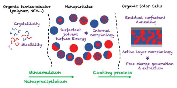
Fig. 2 Scheme of the NP dispersion route to OPV cells
