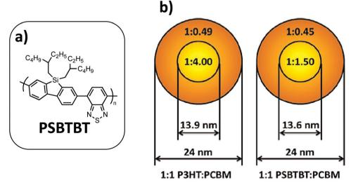
Fig. 16 (a) Chemical structure of PSBTBT. (b) Schematic of small 1:1 P3HT:PC<sub>71</sub>BM and PSBTBT:PC<sub>71</sub>BM NPs showing the core and shell diameters and the polymer: PCBM ratio in the core and shell regions. Adapted with permission from ref. 27 (Copyright 2015 Elsevier B.V.).
