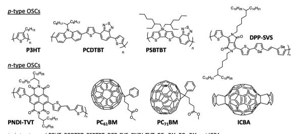
Fig. 5 Chemical structures of P3HT, PCDTBT, PSBTBT, DPP-SVS, PNDI-TVT, PC<sub>61</sub>BM, PC<sub>71</sub>BM and ICBA
