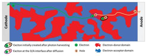
Fig. 1 Typical BHJ scheme for a donor:acceptor blend in organic solar cells.
