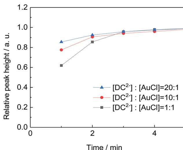
Fig. 7 Comparison of the rate of formation of gold nanoparticles (shown by the height of the absorption peak) by varying the [DC<sup>2-</sup>]:[AuCl] molar ratio at 80 °C. Conditions: [AuCl]: 0.25 mM, [citrate]: 5 mM, pH: 4.4, 80 °C.
