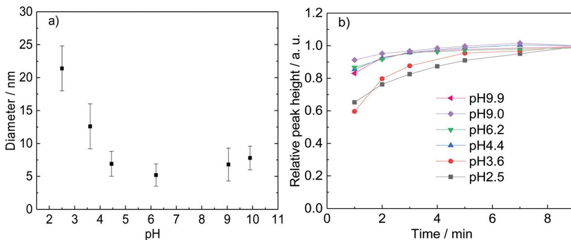
**Fig. 9** Effect of pH on a. Au NP sizes (the error bars represent the standard deviation) and b. rate of formation. Conditions:  $[\text{AuCl}]$ : 0.25 mM,  $[\text{DC}^{2-}]$ : 5 mM,  $[\text{citrate}]$ : 5 mM, 80 °C, time: 7 min–13 min.
