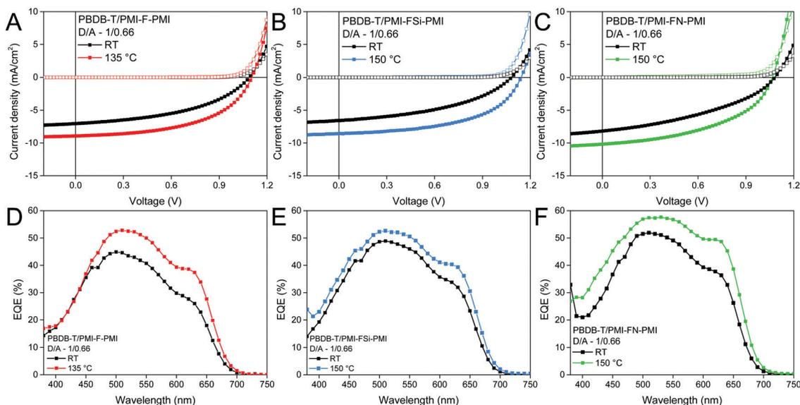
Fig. 7  $J$ - $V$  curves (under illumination – solid symbols and under dark conditions – hollow symbols; notice that the hollow curves overlay) and EQE spectra of the best solar cells of **PBDB-T**: (A and D) **PMI-F-PMI** (**3a**), (B and E) **PMI-FSi-PMI** (**3b**) and (C and F) **PMI-FN-PMI** (**3c**) with a D/A ratio of 1/0.66 w. and w/o annealing of the absorber.
