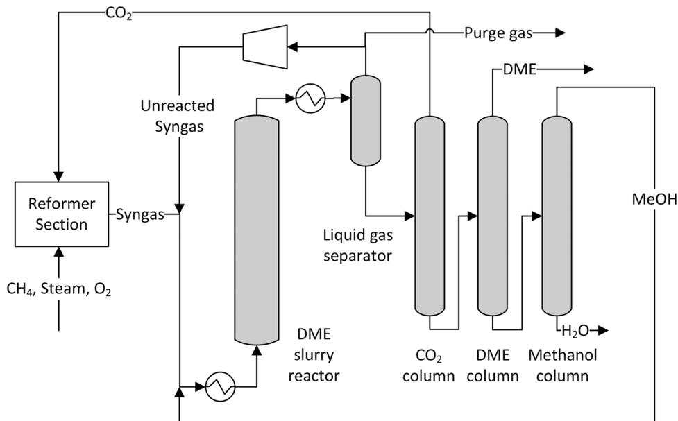
Fig. 16 Schematic process flow of the JFE 100 t per d demonstration plant (own illustration based on Yagi et al.<sup>258</sup>).
