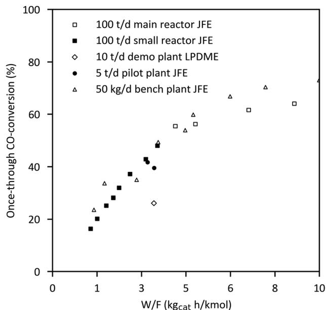
Fig. 17 Dependency of once-through CO conversion on catalyst loading ratio W/F (catalyst weight/reactor inlet gas flow rate) of JFE plants (260 °C, 50 bar)<sup>258</sup> and LPDME 10 t per d demonstration (own calculation based on ref. 261).
