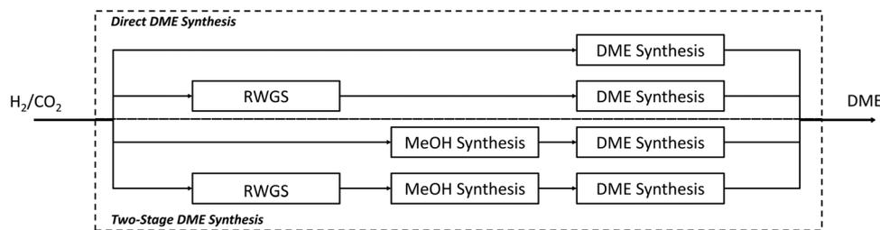
Fig. 19 Possible process pathways from CO<sub>2</sub> to DME.
