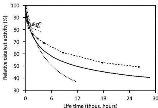
Fig. 5 Deactivation curves of commercial methanol catalysts.<sup>116,117,124,129,130</sup>
