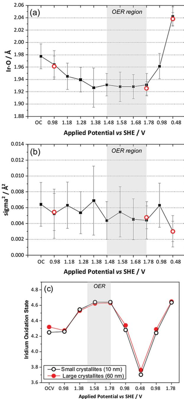
Fig. 4 Plots of EXAFS-derived (a) Ir–O distance, (b) Debye–Waller factor, and (c) comparison of Ir oxidation state from XANES for two particles sizes of  $(\text{Ca}_{0.70}\text{Na}_{0.24})_2\text{Ir}_2\text{O}_6\cdot\text{H}_2\text{O}$  showing also recyclability upon a second oxidation sweep. In (a and b) the red circles are repeated measurements from a second electrode on a later experimental run to check reproducibility. OC = open circuit.
