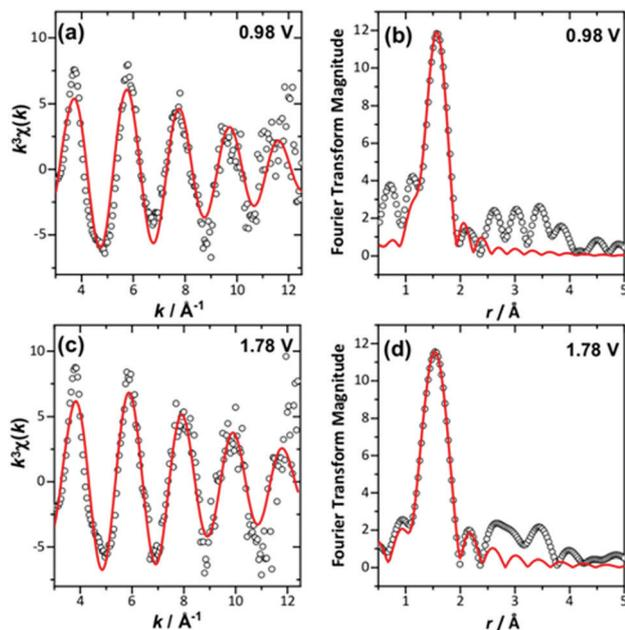
Fig. 3 Single-shell fits of  $k^3$ -weighted EXAFS (left), with Fourier transforms (right) from  $(\text{Ca}_{0.70}\text{Na}_{0.24})_2\text{Ir}_2\text{O}_6\cdot\text{H}_2\text{O}$  at (a) and (b) 0.98 V and (c) and (d) maximum applied potential.
