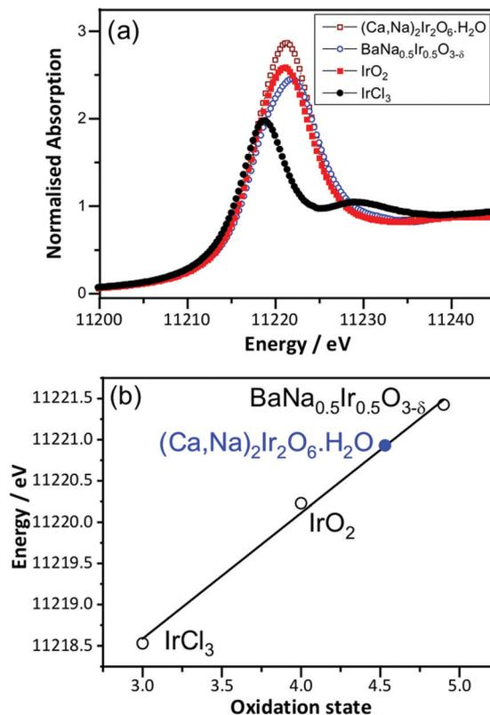
Fig. 2 (a) Room temperature Ir  $L_{\text{III}}$ -edge XANES spectra of  $(\text{Ca}_{0.70}\text{Na}_{0.24})_2\text{Ir}_2\text{O}_6 \cdot \text{H}_2\text{O}$  and reference materials and (b) oxidation state calibration graph, with the white line maximum used.
