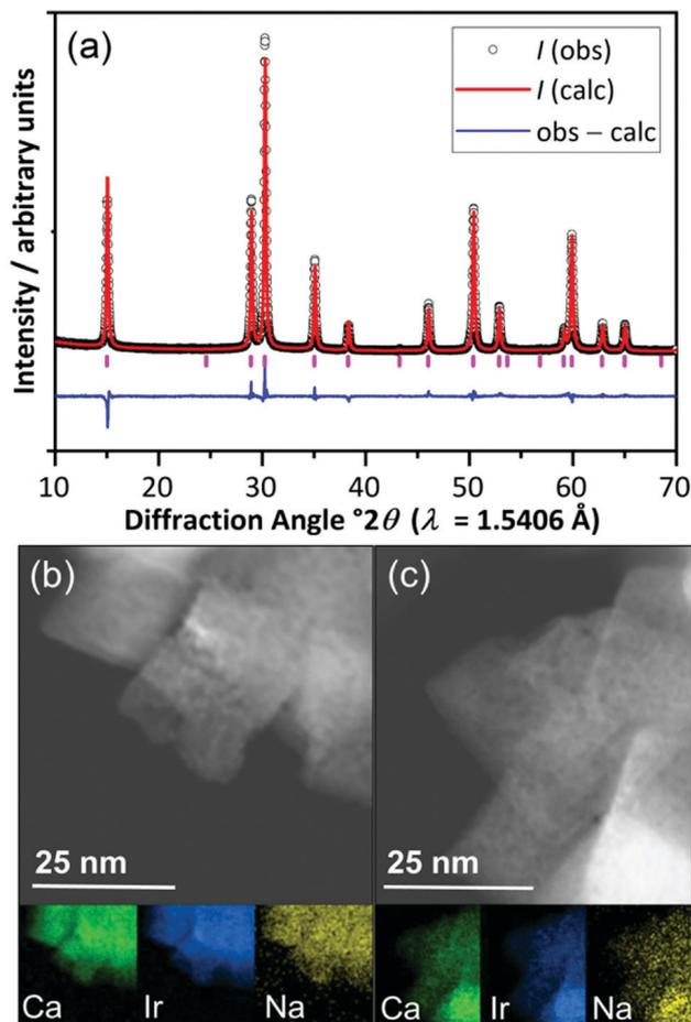
Fig. 1 (a) Rietveld fit to powder XRD of  $(\text{Ca}_{0.70}\text{Na}_{0.24})_2\text{Ir}_2\text{O}_6 \cdot \text{H}_2\text{O}$   $Fd\bar{3}m$ ,  $a = 10.23978(5)$  Å, and (b and c) STEM images and EDXA maps of two regions of the material showing homogeneity of elemental distribution.
