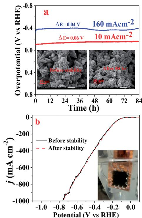
Fig. 8 (a) Chronopotentiometric curve of  $\text{Cuf@Ni}_5\text{P}_4$  at a current density of 10 and  $160 \text{ mA cm}^{-2}$ , inset shows the SEM images obtained before and after the test. (b) LSV of  $\text{Cuf@Ni}_5\text{P}_4$  before and after the chronopotentiometric test.
