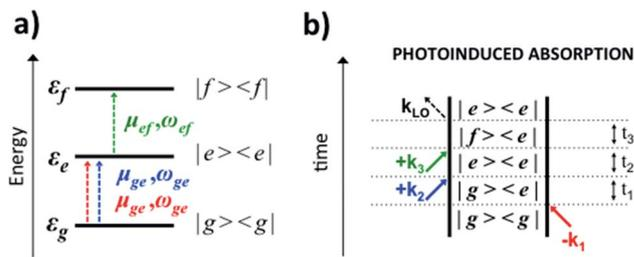
Fig. 4 (a) Scheme of the three-level system, showing transition dipole moments ( $\mu$ ) and frequencies ( $\omega$ ) associated with the ground ( $g$ ) and excited ( $e, f$ ) states and their energies ( $\varepsilon_{g,e,f}$ ). (b) Feynman diagram of a PA signal.
