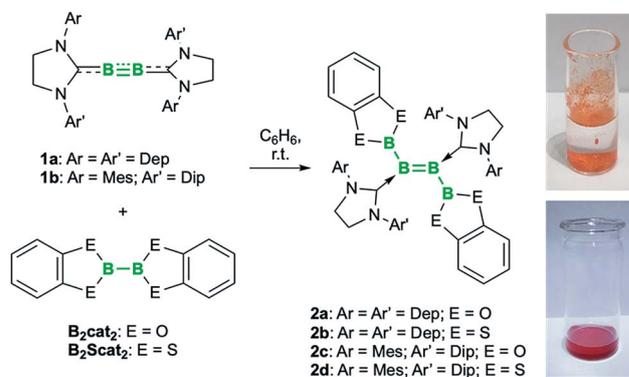
Fig. 2 Catalyst-free diboration of diborynes. Inset photos: suspensions of diborenes **2c** (top) and **2d** (bottom) in water under ambient atmosphere. Dip = 2,6-diisopropyl-phenyl; Dep = 2,6-diethylphenyl.
