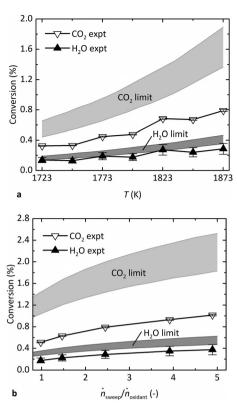
Fig. 4 Comparison of the average experimental conversion of CO<sub>2</sub> and H<sub>2</sub>O at steady state versus equilibrium limits as a function of (a) T, at  $\dot{n}_{\rm sweep}/\dot{n}_{\rm oxidant}$  = 2.4 and 1 Pa O<sub>2</sub>, and (b)  $\dot{n}_{\rm sweep}/\dot{n}_{\rm oxidant}$ , at 1873 K and 0.5 Pa O2.
