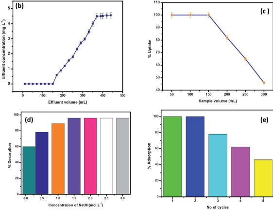
Fig. 7 (a) Diagrammatic representation of column setup for Cr(vI) treatment (b) breakthrough curve (c) effect of sample volume (d) effect of varied NaOH concentrations (e) regeneration efficiency of the biosorbent.
