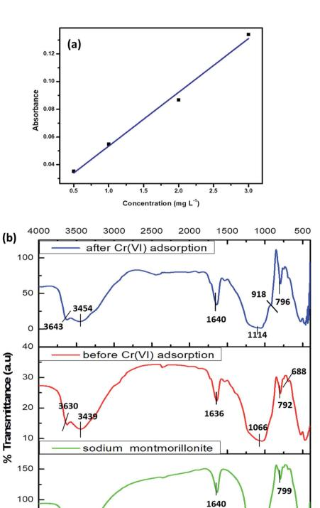
Fig. 1 (a) Calibration graph of Cr(vi) (b) FTIR of sodium montmorillonite, biosorbent before and after Cr(vi) adsorption.
