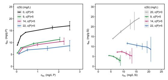
Fig. 3 Simultaneous adsorption of phosphate (left) and silicate (right) onto  $\mu$ GFH with increasing concentrations of silicate (pH 7.0, DI + NaCl); error bars indicate the 95% confidence interval.
