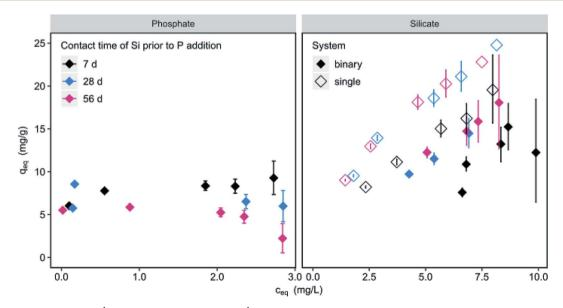
Fig. 6 Phosphate ( $c_0 = 3 \text{ mg L}^{-1}$ ) and silicate ( $c_0 = 10 \text{ mg L}^{-1}$ ) loadings as a function of silicate contact time of 7, 28 and 56 days prior to phosphate addition (filled diamonds) in contrast to silicate as single solute (blank diamonds) ( $c(\mu \text{GFH}) = 150 \text{ mg L}^{-1}$ , pH 7.0, DI + NaCl).
