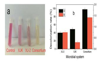
Fig. 4 Decolorization rate of simulated wastewater after 4 days treatment by single *Chlorella sorokiniana* XJK, single *Aspergillus* sp. XJ-2 and the consortium. (a) Decolorization effect of simulated wastewater; (b) decolorization rate and biomass under used different microbial systems (D: decolorization rate; B: biomass).
