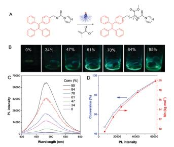
Fig. 8 Visualization of visible light-induced RAFT polymerization. (A) Illustration of the reaction process. (B) Fluorescent photos of the polymer solutions at different conversions taken under 365 nm UV irradiation from a hand-held UV lamp. (C) PL spectra of the polymerization mixtures at different conversions. (D) The exponential relationship of conversion and  $M_n$  with PL intensity. Reproduced from ref. 27 with permission from Wiley-VCH.
