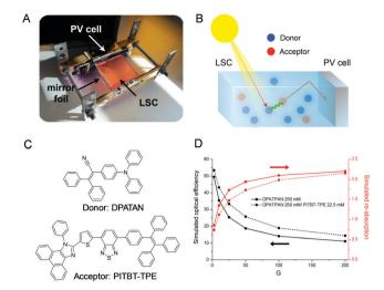
Fig. 18 (A) Setup used for measuring the optical efficiency. (B) Working principle of an ISC with the typical cascade mechanism via FRET by donor and acceptor fluorophores. (C) Chemical structures of DPATAN and PITBT-TPE. (D) Simulated optical efficiencies (black lines) and reabsorption (red lines) of the LSCs as a function of the geometric factor G. Reproduced from ref. 95 with permission from Wiley-VCH.
