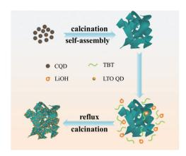
Scheme 1 Illustration of the formation process of LTO QDs/CFs.
