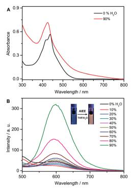
Fig. 4 AIEE behavior of the copolymer. (A) Absorption and (B) emission spectra of copolymer **P(NIPAM-co-EM)** (15.6 μM) in H<sub>2</sub>O/THF mixtures with different  $f_{w}$ ,  $\lambda_{ex}$  = 430 nm; inset (B): fluorescence images of the **P(NIPAM-co-EM)** ( $f_w = 0$  and 90%) under UV light irradiation.
