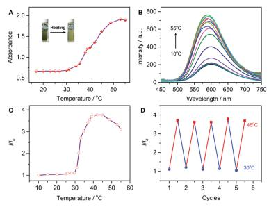
Fig. 5 LCST-featured behavior: (A) temperature-dependent absorption at 430 nm of **P(NIPAM-co-EM)** (14 μM) in an aqueous solution upon heating; inset: images of **P(NIPAM-co-EM)** before and after heating. (B) Temperature-dependent emission spectra of **P(NIPAM-co-EM)** (14 μM),  $\lambda_{ex}$  = 430 nm. (C) The relative fluorescent intensity at 607 nm as a function of temperature. (D) Reversible thermo-response of **P(NIPAM-co-EM)** between 30 and 45 °C by monitoring the fluorescent signal.
