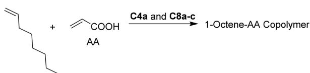
Scheme 6 Copolymerization of 1-octene with acrylic acid catalyzed by \alpha -diimine Pd catalysts. 160
