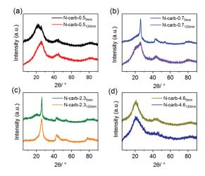
Fig. 4 X-ray diffractrograms for the eight N-doped porous carbon materials produced in the ball mill.
