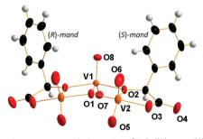
Fig. 3 Molecular structure of the anion  $[V_3O_7((R)-mand)((S)-mand)]^{3-}$ found in 5 showing atom labeling in the central {V3O12} group. Colour code: V orange, O red, C black, and H grey. Displacement ellipsoids are displayed at a 30% probability level.
