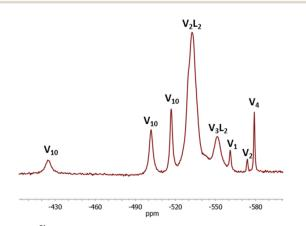
Fig. 4 The  $^{51}$ V NMR spectrum of the NMe $_4$ VO $_3$ -rac-H $_2$ mand-H $_2$ O system,  $c(V) = 0.03 \text{ mol dm}^{-3}$ ,  $c[rac-H_2mand] = 0.02 \text{ mol dm}^{-3}$ , pH = 5.72. Assignment of the chemical shifts:  $V_2L_2 - 533$  ppm,  $V_3L^2 - 551$  ppm,  $V_1 - 561$  ppm,  $V_2 = 574$  ppm,  $V_4 = 579$  ppm, and  $V_{10} = 517$  ppm, -502 ppm and -425 ppm.
