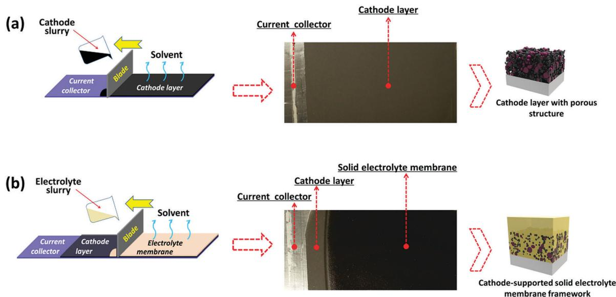
Fig. 2 Fabrication of the cathode-supported solid electrolyte membrane framework. (a) Schematic of the cathode electrode preparation by tape casting, the cathode slurry was tape cast on the aluminium current collector. (b) Schematic of the cathode-supported solid electrolyte membrane preparation by tape casting, the electrolyte slurry was tape cast onto the dry cathode tape showing compact structure after drying.
