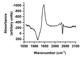
Fig. 6 Difference spectrum in the region 1850-2100 cm<sup>-1</sup> recorded with a pump-probe delay of 1 ns with ground state bleach signal subtracted.
