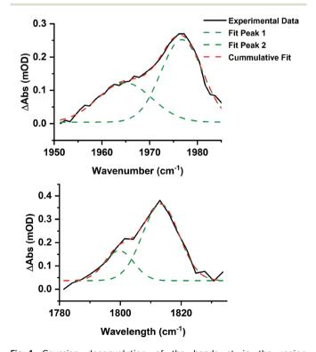
Fig. 4 Gaussian deconvolution of the bands at in the region  $1950-1990~{\rm cm}^{-1}$  (top,  $R^2=0.986$ ) and  $1780-1830~{\rm cm}^{-1}$  (bottom,  $R^2=0.970$ ) at 10 ps. Parameters are listed in Table 1.
