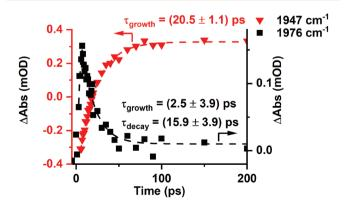
Fig. 5 Change in intensity of the bands due to B (■) and C (▼) with time. Dashed lines show fits against exponential growth/decay (B) and exponential growth (C) kinetics.
