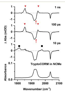
Fig. 3 Bottom IR spectrum of trypto-CORM in NCMe in the region  $1780-2100~{\rm cm}^{-1}$ . Top time-resolved difference IR spectra for the photolysis (400 nm) of trypto-CORM in NCMe with pump-probe delays of 10 ps, 100 ps, and 1 ns showing bands for A and B ( $\blacksquare$ ) and C by ( $\blacktriangledown$ ). The red arrows show the apparent recovery of the GSB for trypto-CORM.
