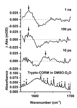
Fig. 9 Bottom IR spectrum of trypto-CORM in DMSO:  $D_2O$  (1:9 v:v) in the region 1560–1700 cm $^{-1}$ . Top time-resolved difference IR spectra for the photolysis (400 nm) of trypto-CORM in NCMe with pump-probe delays of 10 ps, 100 ps, and 1 ns, band positions marked with an arrow. \* indicates bands due to  $H_2O$  contamination.
