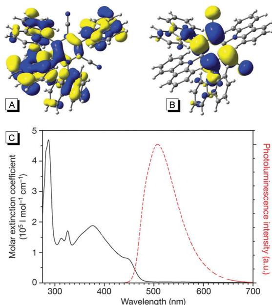
**Fig. 1** (A) HOMOs of 4CzIPN; (B) LUMOs of 4CzIPN; (C) UV-visible and photoluminescence spectra of 4CzIPN. Reprinted in part with permission from ref. 9a. Copyright 2012 Springer Nature Publishers Limited.
