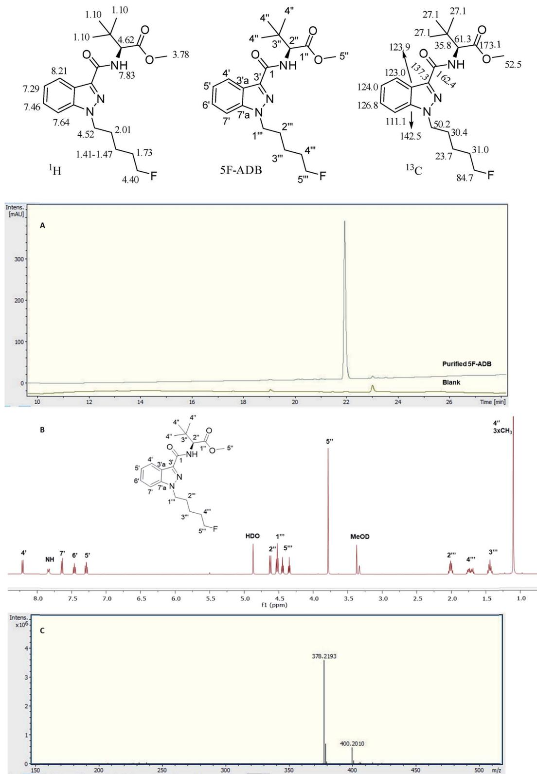
Fig. 2 Analytical purity of 5F-ADB as tested by (A) UHPLC with RT = 22.0 min, (B)  $^1\text{H-NMR}$  in  $\text{CD}_3\text{OD}$  with assignments, and (C) HRMS showing  $[\text{M} + \text{H}]^+$  and  $[\text{M} + \text{Na}]^+$ .
