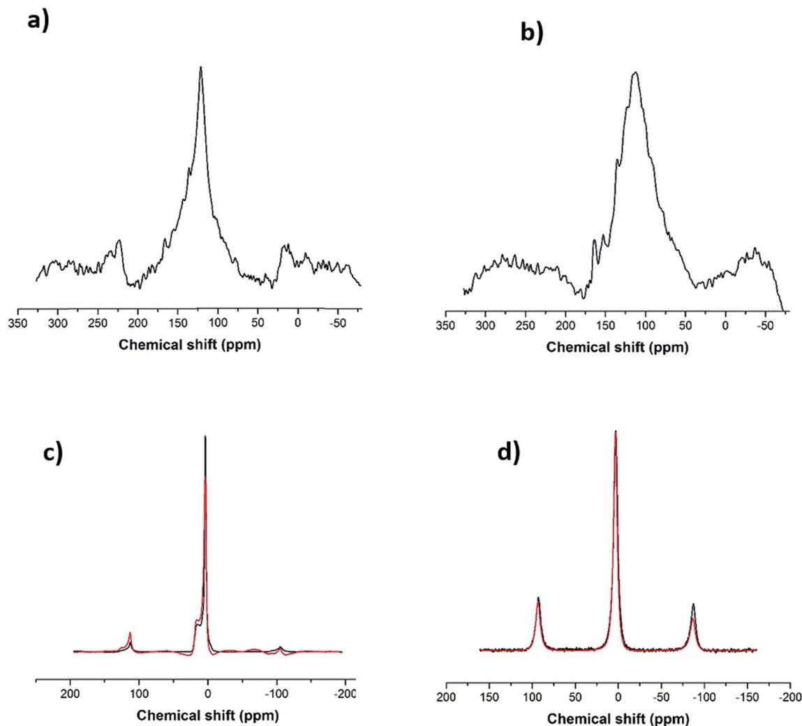
Fig. 3 (a)  $^{13}\text{C}$  SS-NMR spectrum for the as-received SWCNT-1 (the smaller peaks at  $\sim 25$  and  $\sim 225$  ppm are spinning side-bands), (b)  $^{13}\text{C}$  SS-NMR spectrum for the SWCNT-1 mixture residues, (c)  $^{11}\text{B}$  SS-NMR spectra for the fused salt (black line) and the SWCNT-1 mixture residues (red line), (d)  $^7\text{Li}$  SS-NMR spectra for the fused salt (black line) and the SWCNT-1 mixture residues (red line).
