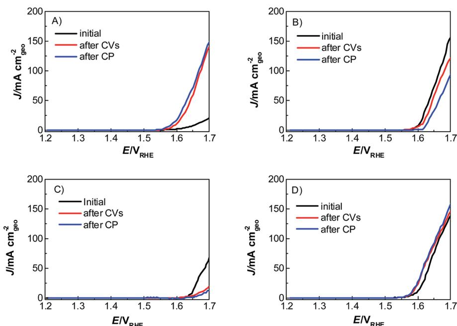
Fig. 3 Linear sweep voltammograms of a commercial mixed oxide  $\text{NiCoO}_2$  catalyst with (A) PIL-1, (B) Nafion, (C) Fumion and (D) no binder from 1.2 to 1.7  $V_{RHE}$  with a sweep rate of  $5 \text{ mV s}^{-1}$ , in 1 M KOH.
