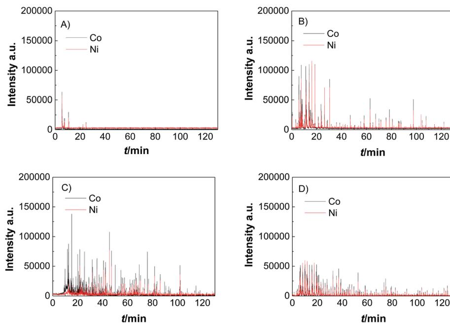
Fig. 5 ICP-OES transient profiles of a commercial mixed oxide  $\text{NiCoO}_2$  with (A) PIL-1, (B) Nafion, (C) Fumion and (D) no binder in 1 M KOH. Corrosion profiles of each catalyst reveal a significantly better stability for the PIL-1 supported catalyst due to fast oxygen bubble removal from the catalyst surface.
