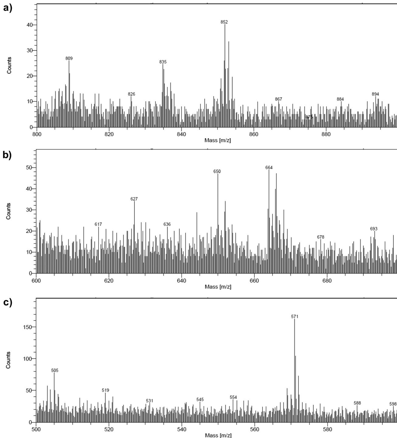
Fig. 6 Positive mode ToF-SIMS spectra of the NiOIRBG-174/CoC<sub>11</sub>P electrode in the  $m/z$  ranges (a) 800–900, (b) 600–700 and (c) 500–600.
