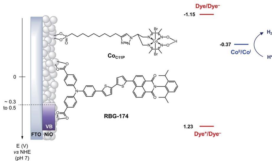
Fig. 1 Schematic energy diagram of the NiOIRBG-174|CoC<sub>11</sub>P photocathode. See text for the estimation of energy levels at pH = 7. Potentials for the redox couples of RBG-174 have been determined as described in ref. 48 from data found in ref. 40.
