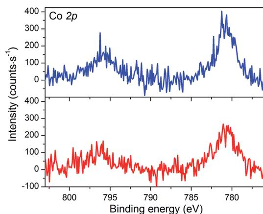
Fig. 4 XPS analyses of the NiO|CoC<sub>11</sub>P (blue line) and NiO|RBG-174|CoC<sub>11</sub>P (red line) electrodes at the baseline-corrected Co 2p core level.
