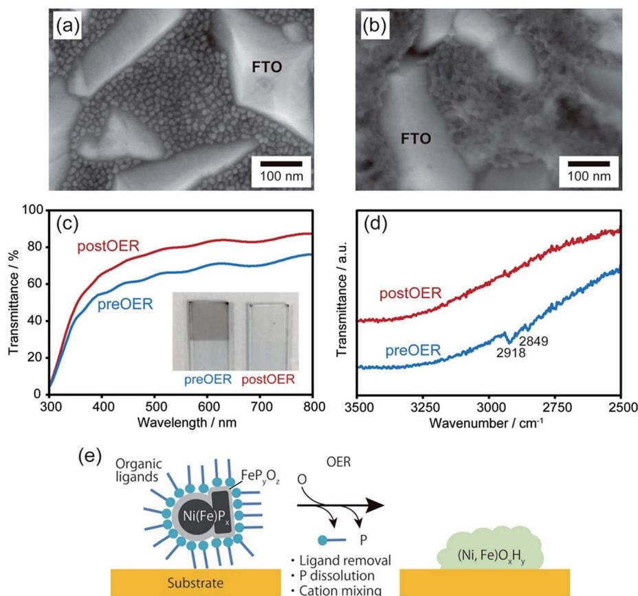
Fig. 3 SEM images of  $\text{NiP}_x@FeP_yO_z$  NP coated FTO glass (a) before and (b) after 30 CV cycles in 0.1 M KOH. (c) Transmittance and (d) FT-IR spectra of  $\text{NiP}_x@FeP_yO_z$  NP coated FTO glass (blue) before and (red) after 30 CV cycles in 0.1 M KOH. The inset in (c) shows the photograph of  $\text{NiP}_x@FeP_yO_z$  NP coated FTO glass. (e) Schematic illustration of the transformation of  $\text{NiP}_x@FeP_yO_z$  NPs into  $(Ni, Fe)O_xH_y$  during the OER.
