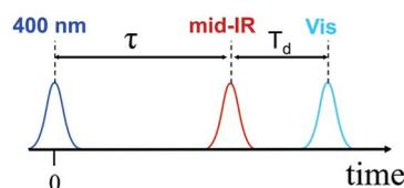
Fig. 1 Pulse sequence used in the 3-pulse experiments.
