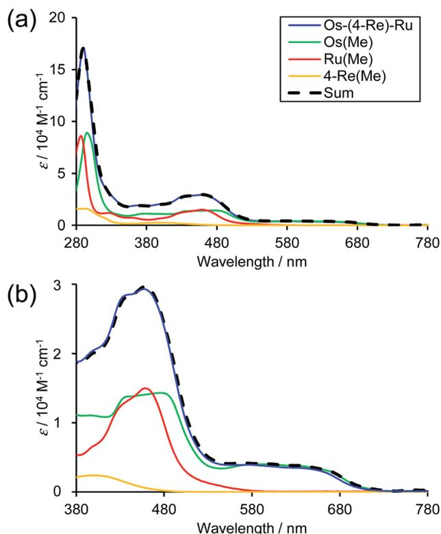
Fig. 3 UV-Vis absorption spectra of the obtained trinuclear complex (a) **Os-(4-Re)-Ru** (blue) and the corresponding mononuclear complexes, *i.e.* **Os(Me)** (green), **Re(Me)** (yellow) and **Ru(Me)** (red). The 1 : 1 : 1 summation spectrum of **Os(Me)**, **4-Re(Me)** and **Ru(Me)** is illustrated as a dotted line. The solvent was MeCN. (b) Enlarged spectra at  $\lambda_{\text{abs}} = 380$  to 780 nm.
