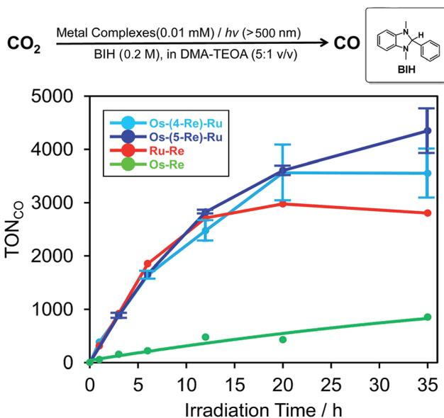
Fig. 7 Time courses of the TON of CO formation during photocatalytic reactions ( $\lambda_{\text{ex}} > 500$  nm) using a mixture of DMA and TEOA (5 : 1 v/v) containing 0.2 M BIH and metal complexes (sky blue: **Os-(4-Re)-Ru**, blue: **Os-(5-Re)-Ru**, red: **Ru-Re**, yellow-green: **Os-Re**). The concentration of each complex was 0.01 mM.
