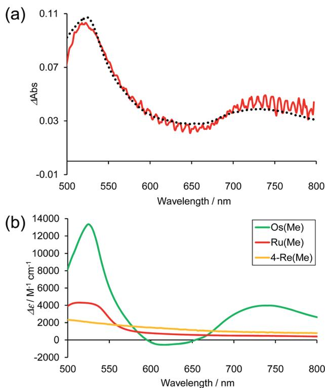
Fig. 10 (a) Difference absorption spectrum of DMA-TEOA (5 : 1 v/v) solution containing **Os-(4-Re)-Ru** (0.01 mM) and BIH (0.1 M) after irradiation at  $\lambda_{\text{ex}} = 480$  nm for 1 min under Ar atmosphere (red line), and the fitting spectrum with 15% **Os(Me)** and 85% **4-Re(Me)** (black line). (b) The difference absorption spectra between the OERS and the non-reduced complexes of **Os(Me)** (green),<sup>10</sup> **Ru(Me)** (red)<sup>40</sup> and **4-Re(Me)** (orange).<sup>40</sup>
