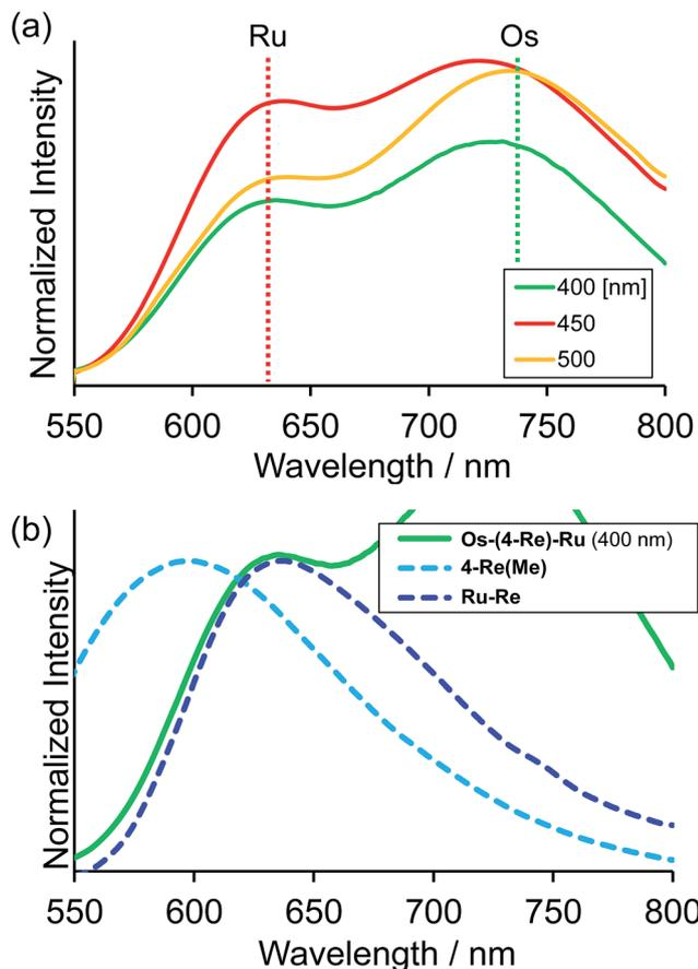
Fig. 4 (a) Emission spectra of Os-(4-Re)-Ru under irradiation at  $\lambda_{\text{ex}} = 400$  nm, 450 nm and 500 nm. The solvent was MeCN. (b) Enlarged emission spectrum of Os-(4-Re)-Ru at  $\lambda_{\text{ex}} = 400$  nm, which is mainly absorbed by the Re unit, with the emission spectra of 4-Re(Me) and Ru-Re.
