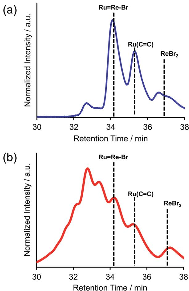
Fig. 1 Size-exclusion chromatogram measured after the reaction to obtain  $\text{Ru}=\text{Re}-\text{Br}$  (a) using  $\text{PPh}_3$  and subsequent air injection and (b) in the absence of  $\text{PPh}_3$ .
