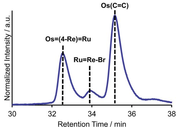
Fig. 2 Size-exclusion chromatogram measured after the reaction for the synthesis of  $\text{Os}=(4\text{-Re})=\text{Ru}$ .
