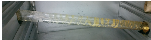
Fig. 6 The helix effect seen as the reaction is occurring on the inner surface of the work-tube. The colour change from colourless to yellow can be seen as the reaction occurs. The opacity of the solution appears to change; this is due to the formation of gas bubbles which are escaping.
