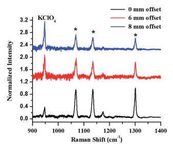
Fig. 8 (a) Raw SORS signals from KClO $_4$  powder filled in 25 mm square HDPE container with a wall thickness of 3 mm with 0 mm (a), 6 mm (b) and 8 mm (c) offsets respectively. Laser beam was focused on to the container. As the offset is increased to 8 mm, the signal of the subsurface material improves.
