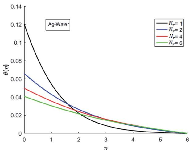
Fig. 24 Temperature curves for various value of  $N_r$  when  $M = 0.5$ ,  $Pr = 0.3$ ,  $Ec = 0.1$ ,  $Gr = 0.5$  and  $\lambda = 1$ .
