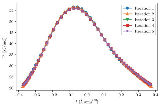
**Fig. 3** Convergence of the ring-polymer instanton at 200 K for H + C<sub>2</sub>H<sub>6</sub>. The initial GPR training set was given by points along the 250 K instanton path. The path length,  $l$ , is defined by eqn (24).
