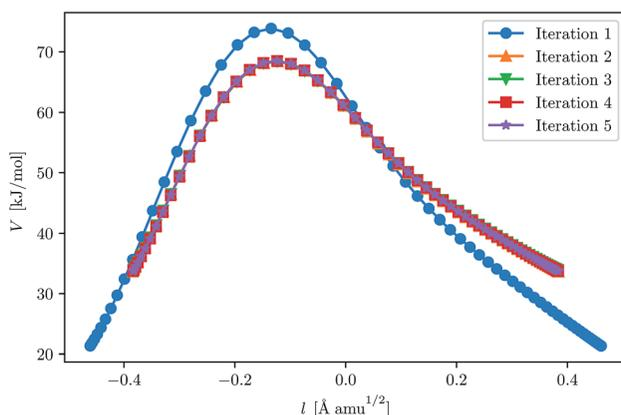
Fig. 2 Convergence of the ring-polymer instanton at 200 K for  $\text{H} + \text{CH}_4$ . The initial GPR training set was defined by eqn (23). The ring-polymer beads are plotted as a function of their potential energy and the path length,  $l$ , as defined by eqn (24).
