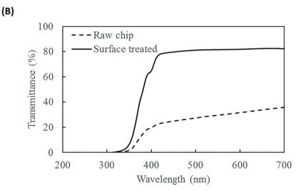
Fig. 3 (A) 3D printed channels at designed sizes of (from left to right) 500 μm, 400 μm, 300 μm, 200 μm, and 100 μm. (B) Light transmittance of the 3D printed chip, with and without rubbing mineral oil onto surface, over 200 to 700 nm wavelength range.
