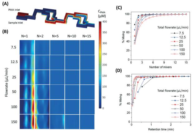
Fig. 2 (A) Demonstration of SAR mixing mechanism: simulated cross-sectional concentration of inlets and the first two mixers at a flowrate of 150 μL min<sup>-1</sup>. (B) Simulated PMA concentration profiles at cross sections after 1, 2, 5, 10, and 15 SAR mixers at flowrates ranging from 7.5 to 150 μL min<sup>-1</sup>. (C and D) Simulated percentage of mixing plotted over number of mixing units passed (C) and total retention time in the mixers (D).
