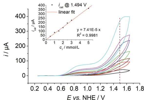
Fig. 4 Concentration dependent CV data of **1** ( $[1] \approx 0.5$ – $5.0$  mM,  $I = 0.1$  M  $\text{PO}_4^{3-}$ , pH = 12,  $\nu = 0.1$  V  $\text{s}^{-1}$ ). Inset: Plot of the catalytic current  $i_c$  at  $E = 1.494$  V vs.  $[1]$ .
