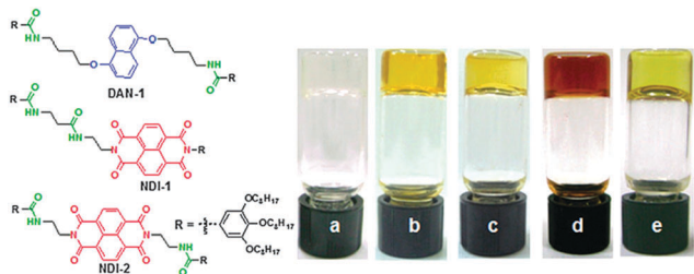
Fig. 3 (left) Structure of the gelators used by Das and Ghosh. 18 DAN-1 and NDI-1 form a self-sorted mixture, whilst DAN-1 and NDI-2 specifically co-assemble. (right) Photos of gels in methylcyclohexane formed by DAN-1 (a), NDI-1 (b), DAN-1 + NDI-1 (c), DAN-1 + NDI-2 (d) and NDI-2 (e). Reproduced from ref. 18 with permission from The Royal Society of Chemistry.
