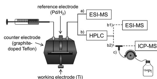
**Fig. 1** Instrumental setup for the electrochemical reduction of Pt(IV) compounds. (a) Species identification by EC-ESI-MS; (b1) EC-LC-ESI-MS or (b2) EC-LC-ICP-MS analysis of Pt(IV) compounds; (c) post-column isotopic dilution analysis for the quantification of Pt species.
