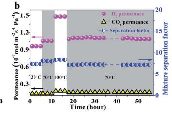
Fig. 4 (a) Mixed gas permeances of different gases through the ZIF-8 membrane prepared on ZnO-modified SSNs at 70  $^{\circ}$ C as a function of kinetic diameter. The inset shows the mixture separation factors. (b) Stability test of ZIF-8 membranes for  $H_2/CO_2$  binary gases.
