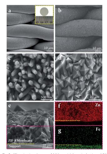
Fig. 2 Microstructure images of (a) bare stainless-steel nets and (b) ZnO nanorods electrodeposited on stainless-steel nets; (c) high magnification view of ZnO nanorods; (d) top view of as-prepared ZIF-8 membrane; (e) cross-sectional images of ZIF-8 membrane; and (f and g) cross-sectional EDXS mapping images of ZIF-8 membrane.
