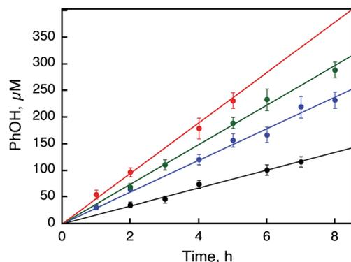
Fig. 6 Time courses of the catalytic hydroxylation of benzene to PhOH with  $\text{H}_2\text{O}_2$  (1.0 mM) in the presence of **1** [10  $\mu\text{M}$  (black), 50  $\mu\text{M}$  (blue), 100  $\mu\text{M}$  (green), and 500  $\mu\text{M}$  (red)] in a solvent mixture of MeCN and  $\text{H}_2\text{O}$  ( $v/v = 23 : 2$ ) containing benzene (1.0 M) and  $\text{Sc}(\text{NO}_3)_3$  (100 mM) at 298 K.
