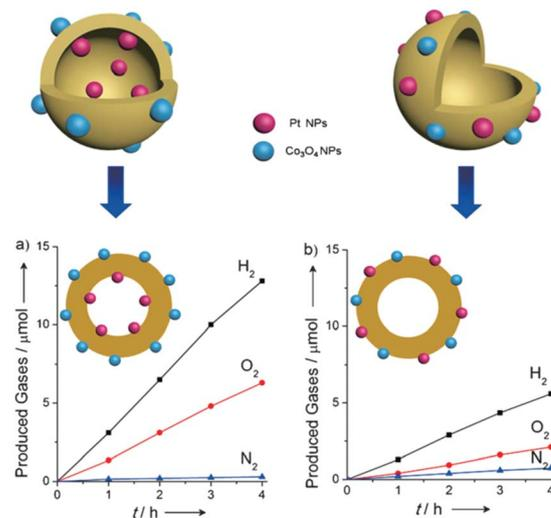
Fig. 13 Time course of the photocatalytic evolution of H<sub>2</sub> and O<sub>2</sub> using (a) Co<sub>3</sub>O<sub>4</sub>/HCNS/Pt and (b) (Co<sub>3</sub>O<sub>4</sub> + Pt)/HCNS under UV irradiation ( $\lambda > 300$  nm). Reprinted with permission from ref. 40. Copyright 2016, Wiley-CVH.
