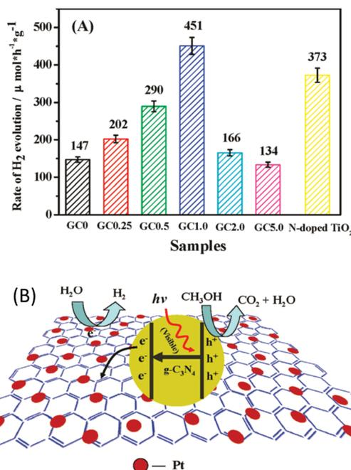
Fig. 9 (A) Comparison of the photocatalytic activities of samples with different loading amounts of graphene on g-C<sub>3</sub>N<sub>4</sub> polymers, (B) proposed mechanism for the enhanced electron transfer process of the graphene/g-C<sub>3</sub>N<sub>4</sub> polymers. Reprinted with permission from ref. 48. Copyright 2011, American Chemical Society.
