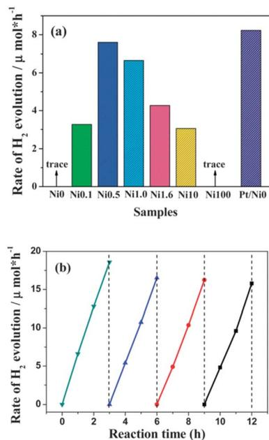
Fig. 7 (a) Comparison of the photocatalytic activity of samples with different amounts of Ni(OH)<sub>2</sub> loaded on g-C<sub>3</sub>N<sub>4</sub> polymers, (b) cyclic H<sub>2</sub>-evolution curve for the Ni0.5 sample. Reprinted with permission from ref. 80. Copyright 2013, Royal Society of Chemistry.
