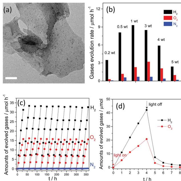
Fig. 12 (a) TEM image of Pt deposited g-C<sub>3</sub>N<sub>4</sub> polymers prepared by *in situ* photo-reduction; (b) overall water splitting activities of g-C<sub>3</sub>N<sub>4</sub> polymers deposited with different amounts of Pt; (c) long reaction time overall water splitting by a Pt-Co-g-C<sub>3</sub>N<sub>4</sub> polymer; (d) overall water splitting activities with the light on and off. Reprinted with permission from ref. 110. Copyright 2016, Royal Society of Chemistry.
