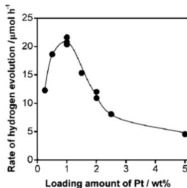
Fig. 4 Dependence of the H<sub>2</sub> evolution rate, when using Pt-loaded g-C<sub>3</sub>N<sub>4</sub> under visible light, on the loading amount of Pt. Reprinted with permission from ref. 56. Copyright 2009, American Chemical Society.
