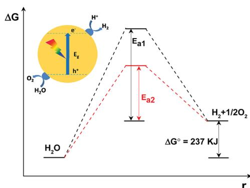
Fig. 2 Schematic description of the energy diagram of a semiconductor modified with both H<sub>2</sub> and O<sub>2</sub> evolution cocatalysts under light irradiation for non-sacrificial photocatalytic water splitting.  $E_{a1}$ : activation energy without cocatalysts;  $E_{a2}$ : activation energy with cocatalysts;  $\Delta G$ : Gibbs free energy change;  $\Delta G^0$ : Gibbs free energy change under standard conditions;  $r$ : redox reaction process.
