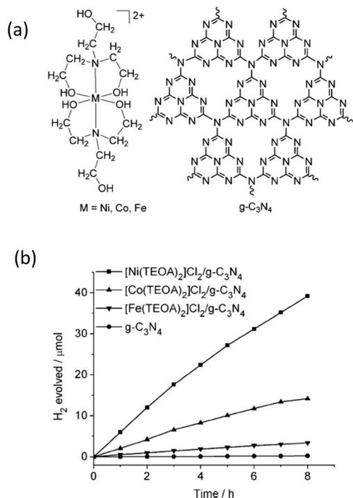
Fig. 8 (a) Structures of Ni-, Co-, and Fe-based cocatalysts and g-C<sub>3</sub>N<sub>4</sub>, (b) photocatalytic H<sub>2</sub>-evolution for different cocatalyst modified g-C<sub>3</sub>N<sub>4</sub> samples. Reprinted with permission from ref. 94. Copyright 2012, Wiley-CVH.
