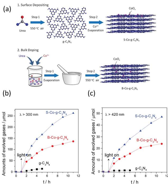
Fig. 11 (a) Schematic illustration of surface modification and bulk doping modification of  $g-C_3N_4$ . Photocatalytic water oxidation activities of the  $g-C_3N_4$ , B-Co- $g-C_3N_4$  and S-Co- $g-C_3N_4$  samples under (b) UV ( $\lambda > 300 \text{ nm}$ ) and (c) visible light ( $\lambda > 420 \text{ nm}$ ) irradiation. Reprinted with permission from ref. 107. Copyright 2016, American Chemical Society.
