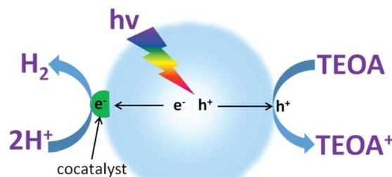
Fig. 3 Schematic illustration of photocatalytic water reduction for H<sub>2</sub> evolution in the presence of an electron donor driven by a semiconductor modified with H<sub>2</sub> evolution cocatalysts. TEOA: triethanolamine.
