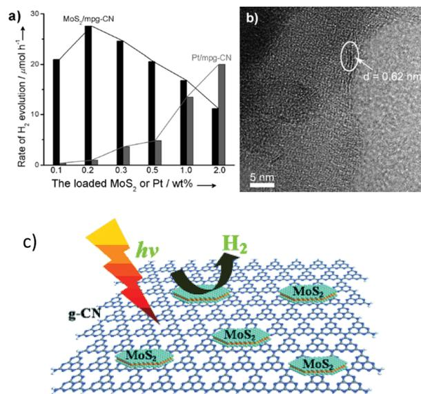
Fig. 6 (a) The rate of H<sub>2</sub> production over mpg-C<sub>3</sub>N<sub>4</sub> loaded with different amounts of MoS<sub>2</sub> or Pt, (b) TEM image of MoS<sub>2</sub>/g-C<sub>3</sub>N<sub>4</sub> and (c) illustration of the deposition of layered MoS<sub>2</sub> on the surface of g-C<sub>3</sub>N<sub>4</sub> for photocatalytic H<sub>2</sub> evolution. Reprinted with permission from ref. 57. Copyright 2013, Wiley-CVH.
