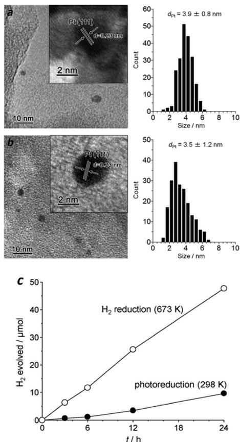
Fig. 5 Size distribution of Pt particles prepared by (a) photoreduction (298 K) and (b) H<sub>2</sub> reduction (673 K); (c) H<sub>2</sub> evolution activities in the presence of an electron donor. Reprinted with permission from ref. 86. Copyright 2014, Royal Society of Chemistry.
