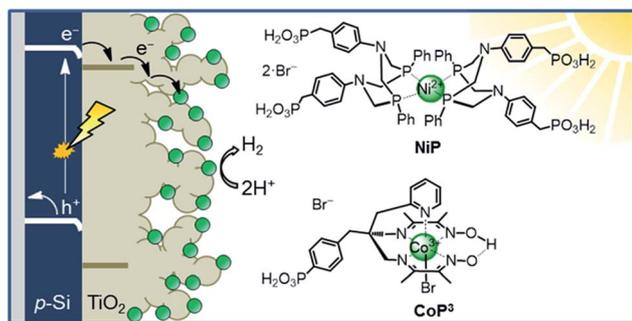
Fig. 1 Schematic diagram of PEC  $\text{H}_2$  evolution with the Si|meso $\text{TiO}_2$ |catalyst photocathode and chemical structures of the immobilised catalysts **NiP** and **CoP<sup>3</sup>**.
