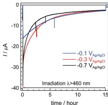
Fig. 6 Time courses of the photocurrent using the RuRe/CuGaO<sub>2</sub> photocathode at various potentials (corresponding to entries 1–3 in Table 1) under irradiation at  $\lambda_{\text{ex}} > 460$  nm.
