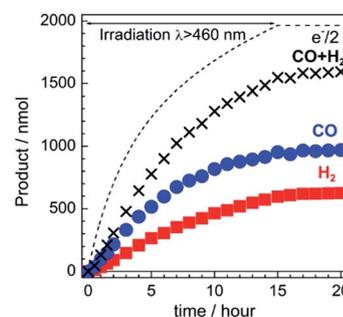
Fig. 4 Time courses of the chemical products ( $\text{CO}$  and  $\text{H}_2$ ) and a half amount of electrons passing through the **RuRe/CuGaO<sub>2</sub>** photocathode under continuous visible-light irradiation ( $\lambda_{\text{ex}} > 460$  nm) at  $-0.3$  V vs. **Ag/AgCl**. A 50 mM aqueous solution of  $\text{NaHCO}_3$  (pH 6.6) that was saturated with  $\text{CO}_2$  was used as the electrolyte.
