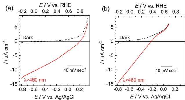
Fig. 1 Current-potential curves of **RuRe/CuGaO<sub>2</sub>** (a) and **RuRe/NiO<sup>31</sup>** (b) electrodes under continuous visible-light irradiation ( $\lambda_{\text{ex}} > 460$  nm) and under dark conditions. A 50 mM aqueous solution of  $\text{NaHCO}_3$  (pH 6.6) saturated with  $\text{CO}_2$  was used as the electrolyte.
