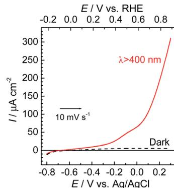
Fig. 7 Current–potential curves of the CoO<sub>x</sub>/TaON photoanode under continuous visible-light irradiation ( $\lambda_{\text{ex}} > 400$  nm) and under dark conditions. A 50 mM aqueous solution of NaHCO<sub>3</sub> (pH 6.6) saturated with CO<sub>2</sub> was used as the electrolyte.
