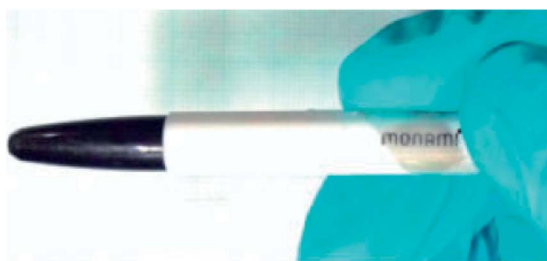
Fig. 22 Fully rollable graphene-based NG. 103
