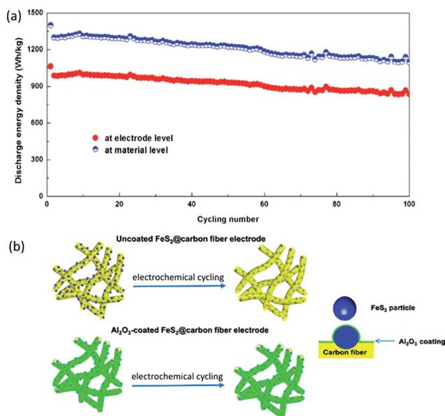
Fig. 13 (a) Cycling stability at material level ( $\text{W h kg}_{\text{FeS}_2}^{-1}$ ) and electrode level ( $\text{W h kg}_{\text{FeS}_2 \text{ electrode}}^{-1}$ ) for  $\text{Al}_2\text{O}_3$ -coated  $\text{FeS}_2@\text{carbon fiber}$  electrode; (b) illustration of mechanisms for the enhanced cycling stability by  $\text{Al}_2\text{O}_3$  coating. Reproduced with permission from ref. 180, copyright 2016, American Chemical Society.
