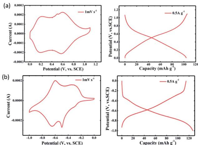
Fig. 15 CV and charge/discharge curves (0.5 A g<sup>-1</sup>) for (a) polytriphenylamine cathode, (b) 1,4,5,8-naphthalenetetracarboxylic dianhydride-derived polyimide anode. Reproduced with permission from ref. 186, copyright 2017, John Wiley and Sons.
