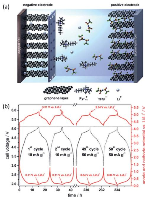
**Fig. 17** (a) Schematic illustration of a dual-ion battery using graphite as both cathode and anode, with the formation of a stable SEI layer at the negative graphite electrode. (b) Cathode potential, anode potential (red curves) and cell voltage (dotted black curve) profiles. Reprinted with permission.<sup>193</sup>
