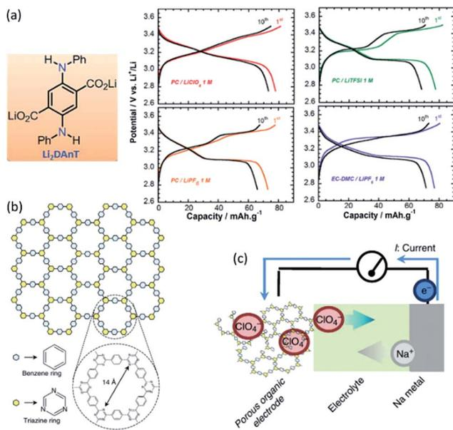
Fig. 18 (a) Structure of Li<sub>2</sub>DAnT and voltage profiles of Li<sub>2</sub>DAnT when hosting different anions.<sup>197</sup> (b) Porous organic anion host of having a honeycomb structure with a pore diameter of 1.4 nm, and (c) discharging process with ClO<sub>4</sub><sup>-</sup> anions move out from the organic host. Reproduced with permission from ref. 198, copyright 2013, Nature Publishing Group.
