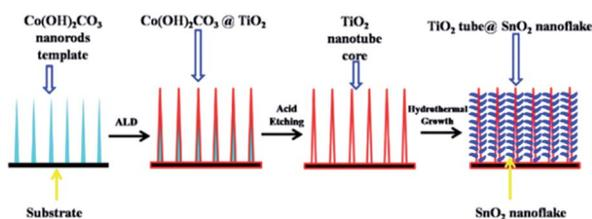
Fig. 9 Schematics of the fabrication process of TiO<sub>2</sub> nanotube@SnO<sub>2</sub> nanoflake core-branch nanostructures. Reproduced with permission from ref. 134, copyright 2014, Elsevier.
