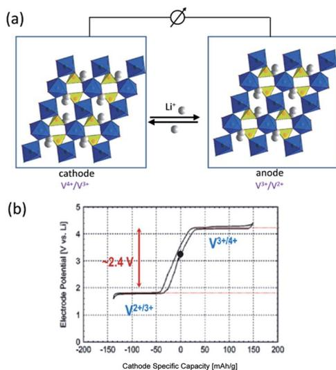
Fig. 19 (a) Schematic illustration of a symmetric LIB with two redox couples of V<sup>4+</sup>/V<sup>3+</sup> and V<sup>3+</sup>/V<sup>2+</sup> in the LiVPO<sub>4</sub>F. Reproduced with permission from ref. 201, copyright 2011, American Chemical Society. (b) (De)lithiation reactions for a Li/LiVPO<sub>4</sub>F cell from 1.6 to 4.4 V showing two potential steps with a gap of about 2.4 V. Reproduced with permission from ref. 202, copyright 2013, American Chemical Society.
