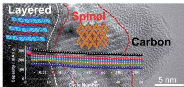
Fig. 11 A Li-rich LSC heterostructured cathode material, comprised of a Li-rich layered core, a spinel interlayer, and a carbon nanocoating. Reproduced with permission.<sup>158</sup>
