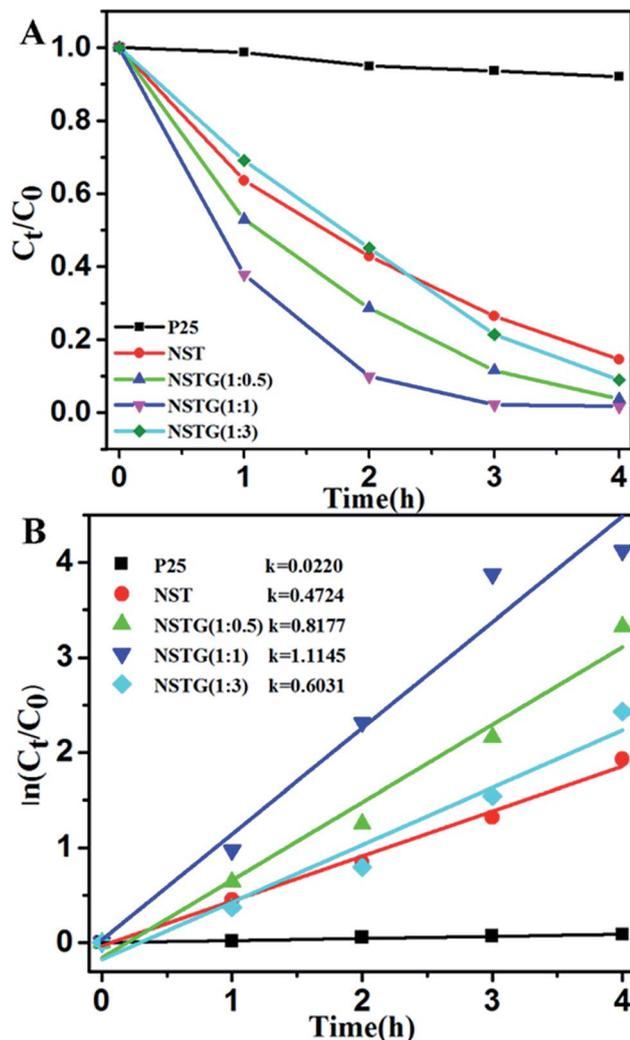
Fig. 7 (A) Photocatalytic activities and (B) linear fittings of the pseudo-first order kinetics model for the degradation of methylene blue (MB) under visible light ( $\lambda > 400$  nm) irradiation for the different catalysts: P25, NST, NSTG(1 : 0.5), NSTG(1 : 1) and NSTG(1 : 3).
