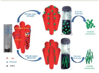
Fig. 28 Proposed mechanism for the formation of 0-D and 1-D polyaniline (PANI) nanostructures in swollen liquid crystals (SLCs).77 Reproduced with permission from Wiley-VCH.
