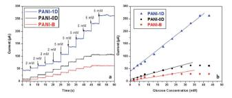
Fig. 36 (a) Chronoamperometric response of polyaniline (PANI) nanostructures synthesized using swollen liquid crystals (SLCs) and bulk polyaniline (PANI) with varying concentration of glucose in PBS buffer (pH = 7.2) (b) calibration curves corresponding to the chronoamperometric glucose detection. Adapted with permission from ref. 90, copyright 2015, Biointerface Research in Applied Chemistry.
