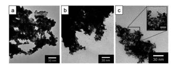
Fig. 8 TEM images of Bi nanoparticles produced by shear mixing of lyotropic liquid crystals (LLCs) (a) hexagonal phase (b) lamellar phase (c) inverse hexagonal phase. Reprinted with permission from ref. 32. Copyright 2004 American Chemical Society.
