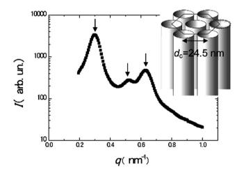
Fig. 14 Small angle X-ray scattering (SAXS) spectrum of the Pd–Au doped hexagonal mesophase and scheme of the structure of the mesophase. The arrows point to the three main peaks. Reprinted with permission from ref. 59. Copyright 2009 American Chemical Society.
