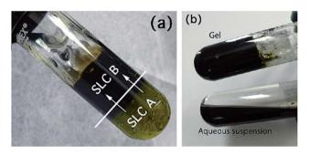
Fig. 25 Synthesis of polypyrrole (PPy) nanoparticles in lamellar swollen liquid crystals (a) using swollen liquid crystals (SLCs) containing the pyrrole (A) and the swollen liquid crystals (SLCs) containing ammonium peroxydisulfate (B); (b) product at end of reaction (top) and polypyrrole (PPy) nanoparticles obtained after extraction (bottom). Reprinted with permission from ref. 80. Copyright 2010 American Chemical Society.
