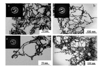
Fig. 18 TEM images of palladium nanowires formed in hexagonal mesophases using electron beam irradiation with different cosurfactant: surfactant ( $n_{\rm cosurfactant}$ :  $n_{\rm surfactant}$ ) molar ratio (a) 0.78 (b) 0.85 (c and d) 0. Reprinted with permission from ref. 72. Copyright 2009 American Chemical Society.
