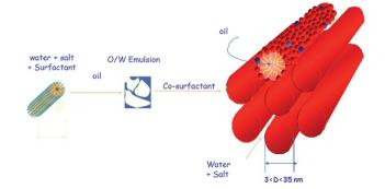
Fig. 10 Formation of swollen hexagonal mesophase from a four component system: water, surfactant, oil and cosurfactant.
