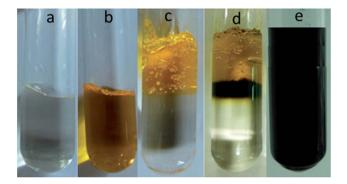
Fig. 31 Photographs of (a) mesophase containing aniline, (b) mesophase containing gold chloride, (c) mesophases at the time of mixing, (d) mesophases after 1 h reaction and (e) mesophases after 72 h showing the completion of reaction. Reproduced from ref. 83 with permission from the Centre National de la Recherche Scientifique (CNRS) and The Royal Society of Chemistry.
