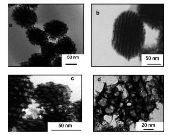
Fig. 21 TEM images of porous platinum nanoballs made by connected nanowires and formed after complete reduction (16 h  $\gamma$ -irradiation) dose rate 3 kGy h<sup>-1</sup>. Reprinted with permission from ref. 58. Copyright 2007 American Chemical Society.
