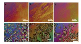
Fig. 11 Room temperature crossed polarizing optical microscopy (POM) optical images of (a-c) fresh mesophases containing aniline, aniline hydrochloride and  $H_2PtCl_6 \cdot 6H_2O$  respectively, (d-f) fan shaped focal conic texture in the same samples after 48 hours. Reproduced from ref. 52 with permission from Elsevier.
