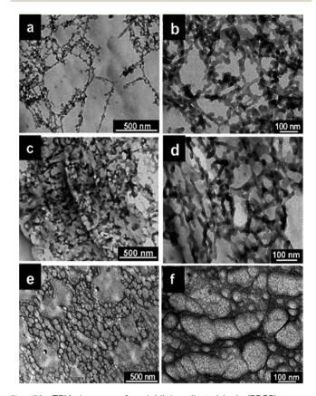
Fig. 30 TEM images of poly(diphenylbutadyine) (PDPB) nanostructures prepared using UV irritation in mesophases with (a and b)  $\phi$ (swelling ratio), volume ratio of oil over water (v/v) = 2.21 and  $C_s$  (total salt concentration) = 0.3 M NaCl, (c and d)  $\phi$  = 0.98 and  $C_s$  = 0.1 M NaCl, (e and f)  $\phi = 0.72$  and  $C_s = 0$  M NaCl. Reproduced from ref. 82 with permission from the Centre National de la Recherche Scientifique (CNRS) and The Royal Society of Chemistry.
