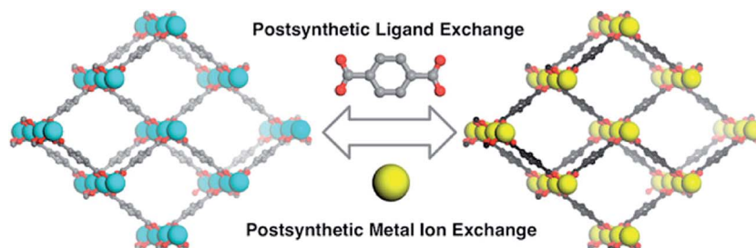
Fig. 2 Post-synthetic ligand and metal ion-exchange (PSE) processes. Reproduced with permission from ref. 42, copyright 2012, American Chemical Society.
