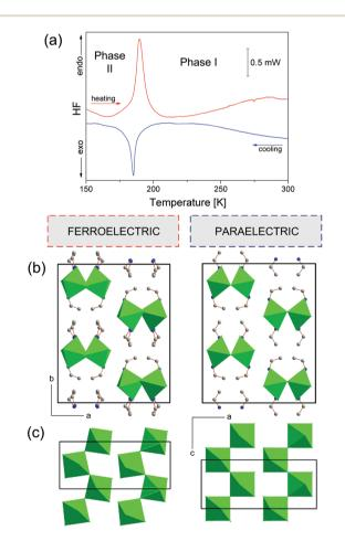
Fig. 1 (a) DSC data confirming the transition sequence seen in ECB (rate: 10 K min<sup>-1</sup>, sample mass: 12.86 mg); (b) the structure overview of the paraelectric Phase I (right) and ferroelectric Phase II (left); (c)  $[BiCl_5]^{2-}$  chains propagate along the c-direction and distinctly deform after the PT.
