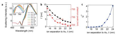
Fig. 3 Plasmonic tuning of scattering and SERS by applied potential. (a) Simulated plasmonic response (COMSOL) of 80 nm NPoM with 1.5 nm shell with refractive index from n=1 (blue) to n=1.33 (red). Overall shift  $\Delta\lambda\sim15$  nm. (b) Calculated peak width  $\Gamma$  due to Drude damping (black), and calculated coupled plasmon peak wavelength (red), vs. ion separation to gold. (c) Quality factor of plasmonic resonance,  $Q^4$ , vs. ion separation to gold.
