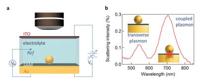
Fig. 1 Opto-electrochemistry and SERS detection. (a) Optically transparent thin (sub-mm) electrochemical cell for spectroscopy of single 80 nm Au NPs on molecular layer on Au. Potential  $V_{\rm s}$  applied between ITO working electrode and Au counter-electrode, with a Pt wire pseudo-reference electrode ( $V_{\rm m}$ ). (b) Typical scattering spectrum of single 80 nm Au NPoM with biphenyl-4-thiol (BPT) spacer.
